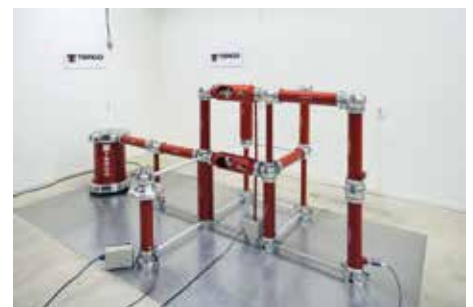
2-stage Impulse Voltage Test Set-up
