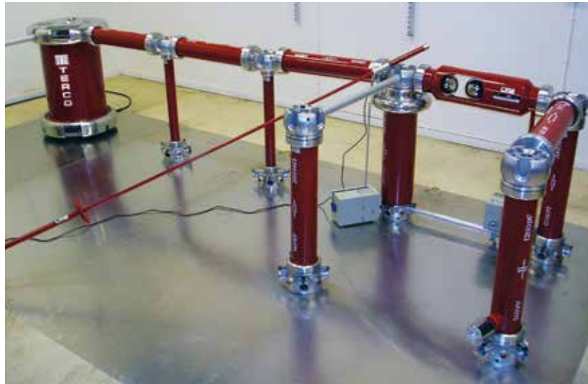
Single-stage Impulse Voltage Test Set-up Discharger Rod on the Capacitor
