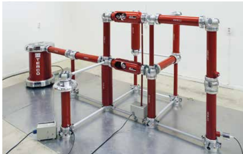
2-stage Impulse Voltage Test Set-up
