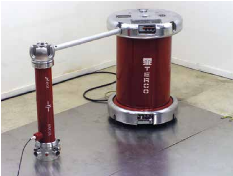
Single-stage AC Voltage Test Set-up
