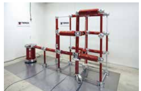
3-stage DC Voltage Test Set-up
