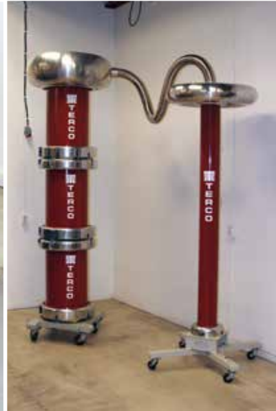
3-stage AC Voltage Test Set-up
