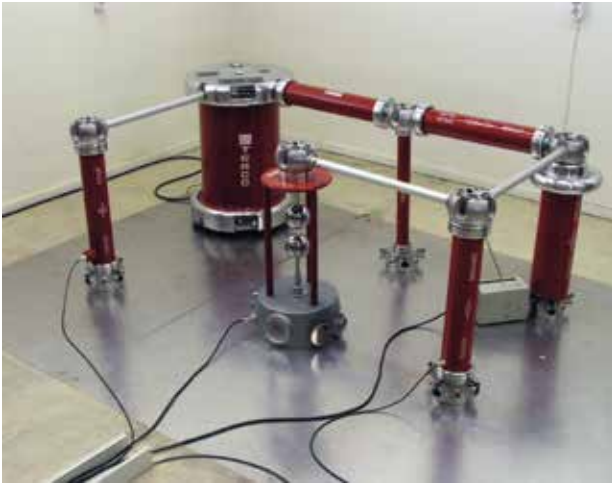
Measurement of flashover
