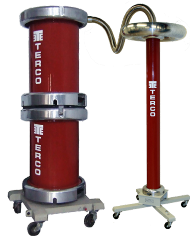
2-stage AC Voltage Test Set-up
