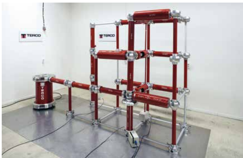
3-stage Impulse Voltage Test Set-up
